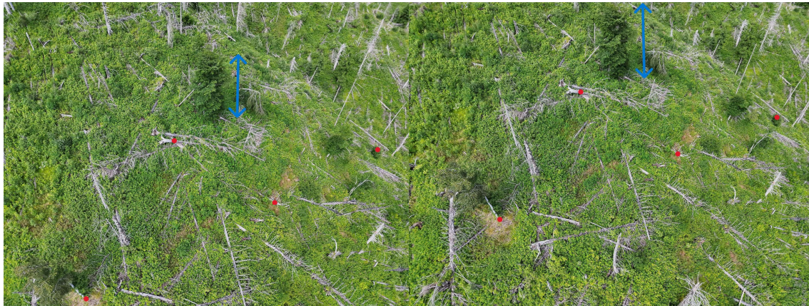
Fig. 1: Successive pictures shot by UAS. In red, possible tie points (managed internally by the software). In blue, the difference in tree height between pictures-tree length, in 2D-enables its 3D reconstruction.
