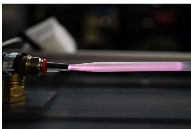
Figure 14 Plasma discharge generated by the CaviPlasma system, producing reactive species for water sanitation and micropollutant degradation.
