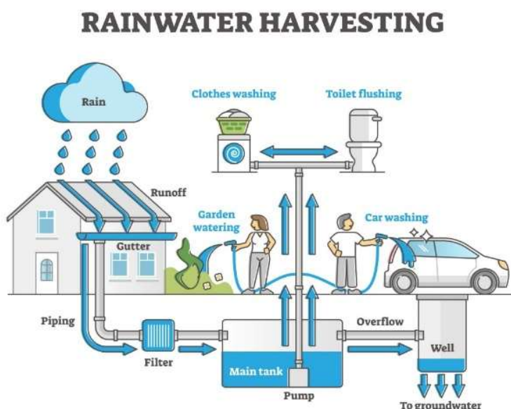
Figure 3: Rainwater harvesting diagram - conventional ( allamericangutterprotection.com .)
