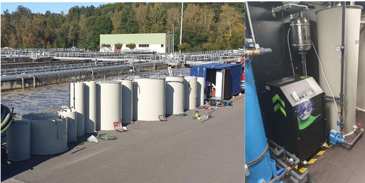
Figure 12 Ozonation process applied to treated effluent from a wastewater treatment plant (WWTP Liberec, Czechia).
