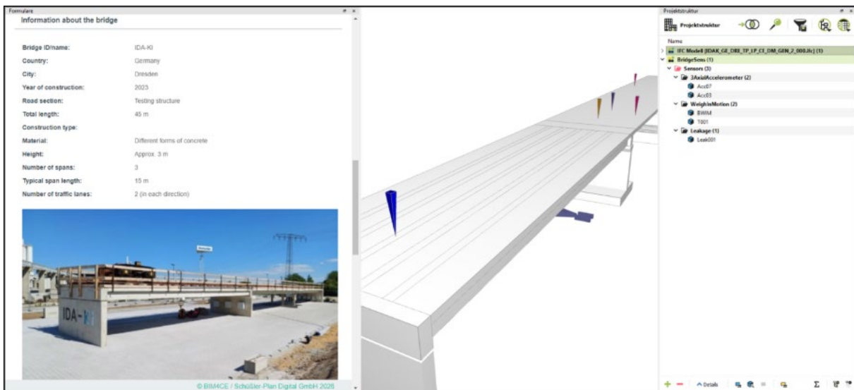
Figure 34. General bridge information visualized on the DT platform for openLAB Bridge
