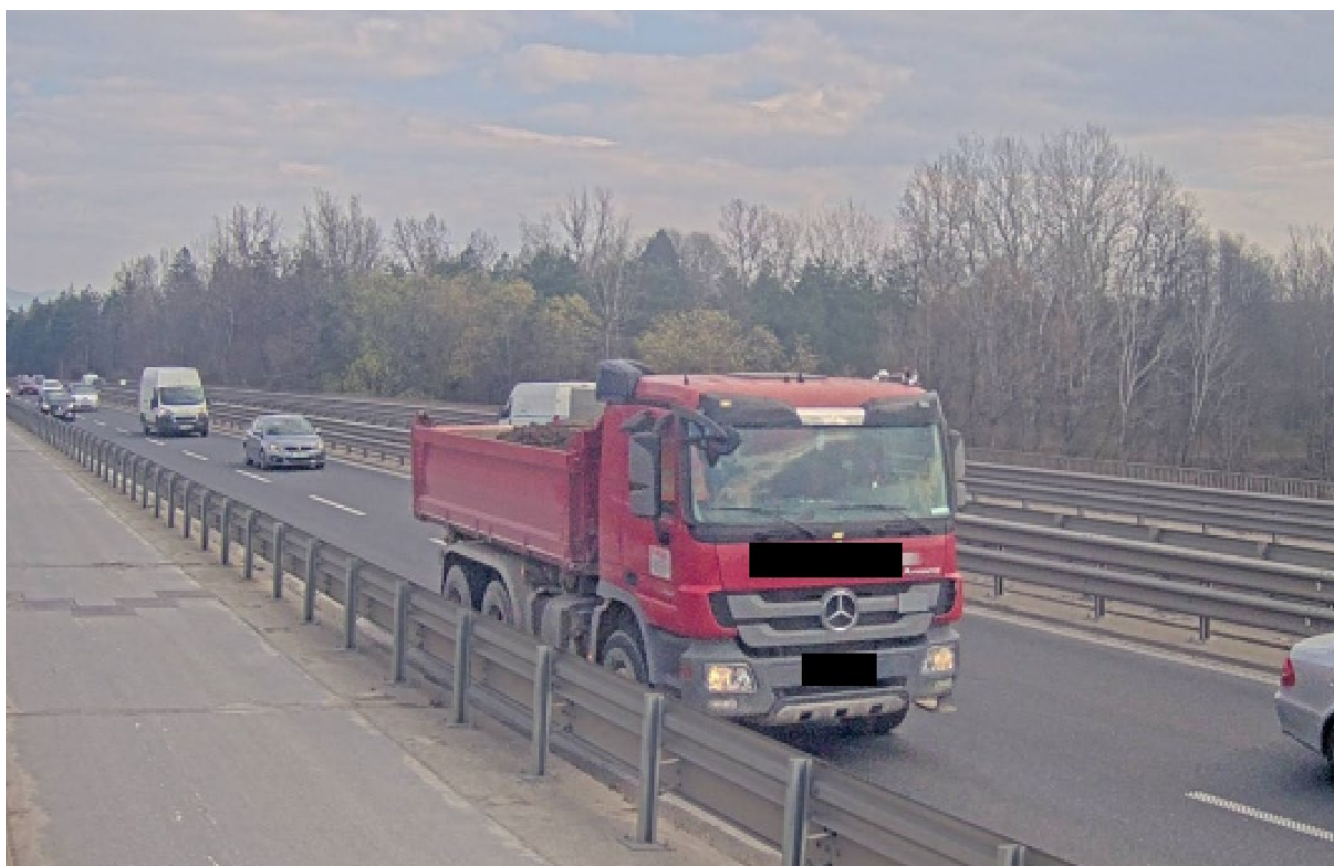
Figure 50. A typical 3-axle vehicle carrying construction material
