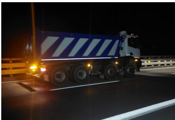
Figure 20. Dynamic load test on Sant'Ambrogio bridge
