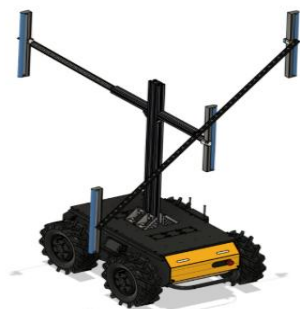
Figure 2. (a) CAD design and (b) laboratory prototype of the autonomous UV-C robotic platform developed for photonic pest management in vineyards.
