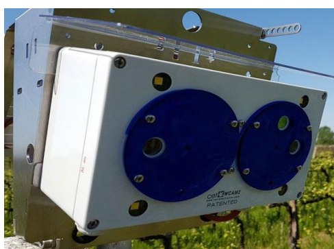
Figure 8. WCAM stereo-imaging system used for vineyard canopy monitoring.
