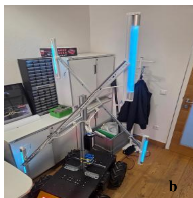
Figure 2. (a) CAD design and (b) laboratory prototype of the autonomous UV-C robotic platform developed for photonic pest management in vineyards.
