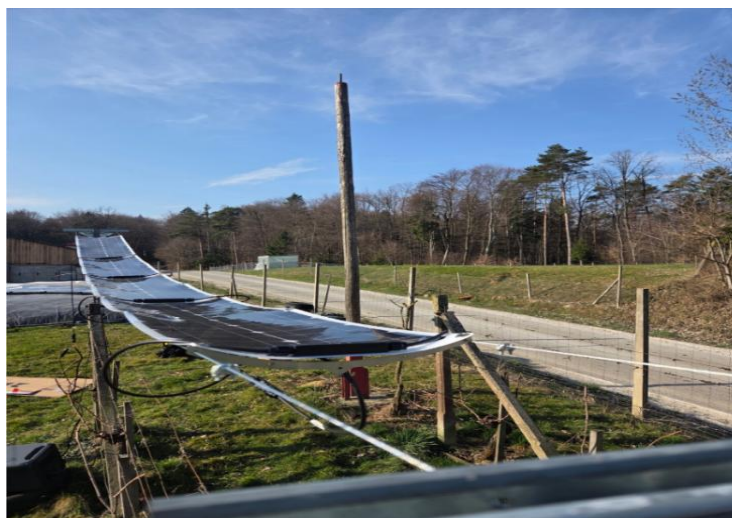
Figure 1. Agrivoltaic vineyard infrastructure prototype developed for solar-energy harvesting, rainwater collection, and precision irrigation applications
