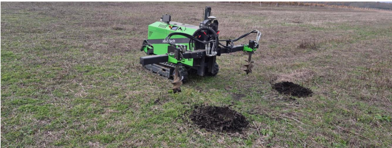
19. Figure: Robot drilling holes at the pilot site
