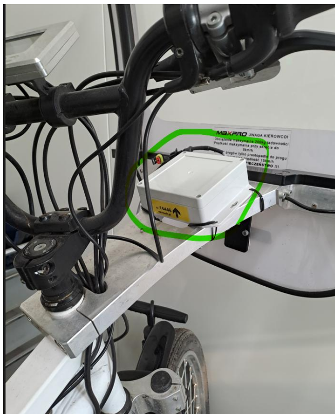
Figure 7 GPS sensor placed on bike construction (source: own photo)
