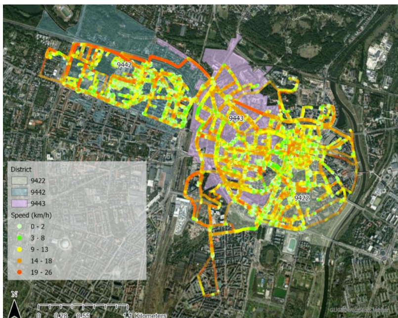
Figure 12 Average speed “zones” of cargobikes (GPS data)
