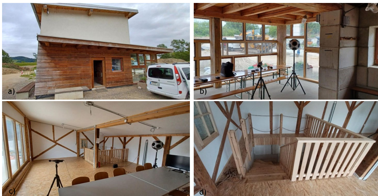
Figure 1: Photos during initial measurements without panels installed. outside of pilot building (a); ground floor meeting room (b); upstairs conference room (c) and open staircase between floors (d)
