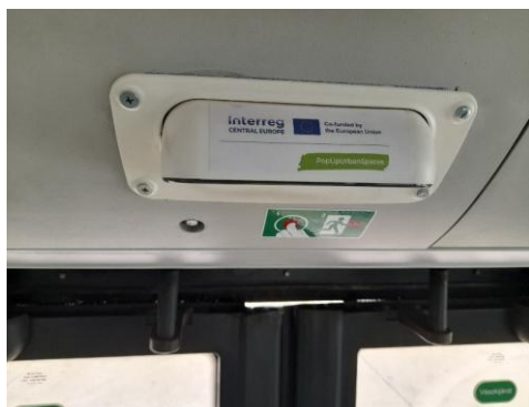
Sensors are placed above passenger entrances to the bus. Credits: MÁV Passenger Transport Co.
