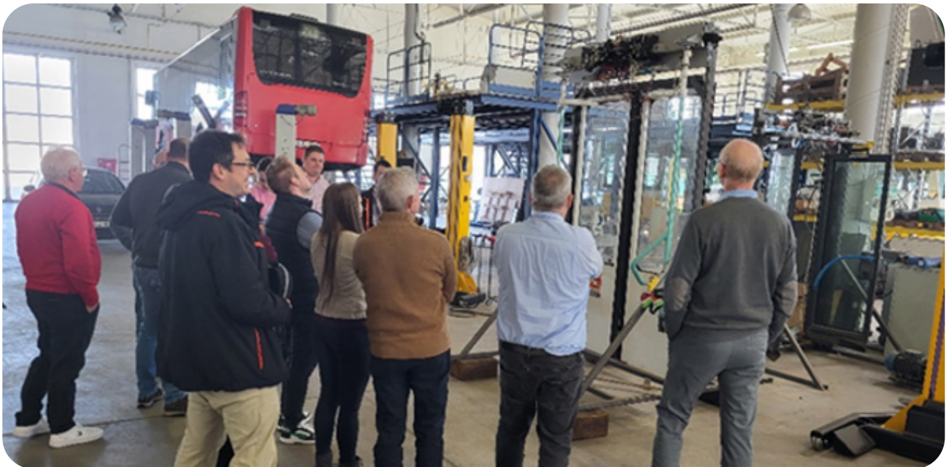
Figure 30: Controlled test environment used for functional testing of the newly developed door control unit.
