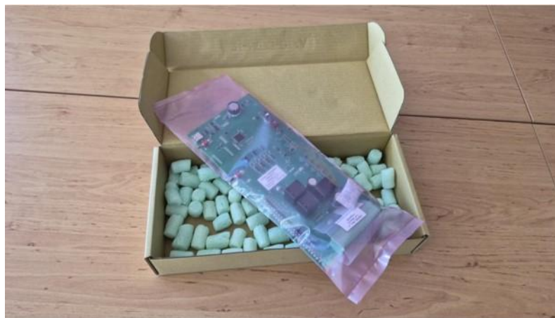
Figure 5 One of the 40 new door control units produced within the pilot action in Szeged
