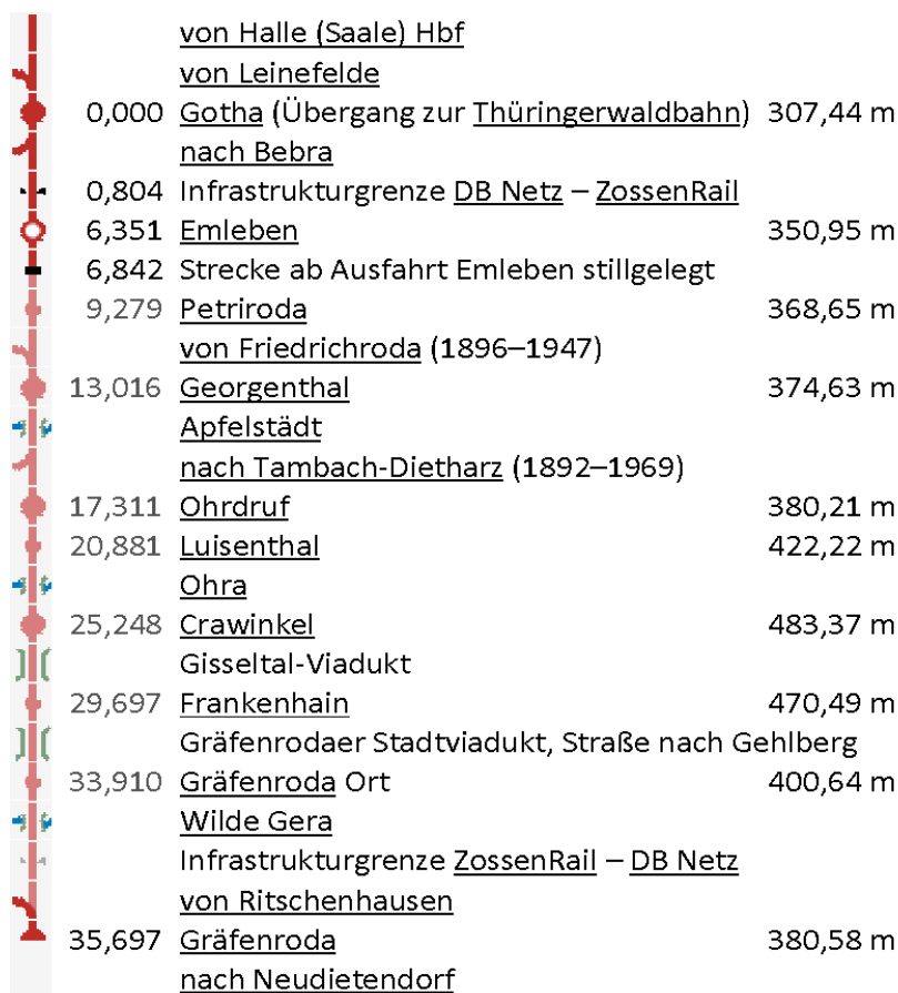
Fig.5. Railway line between Gotha and Gräfenroda with stations, distances and elevation profile; decommissioned sections are indicated in grey/light red
