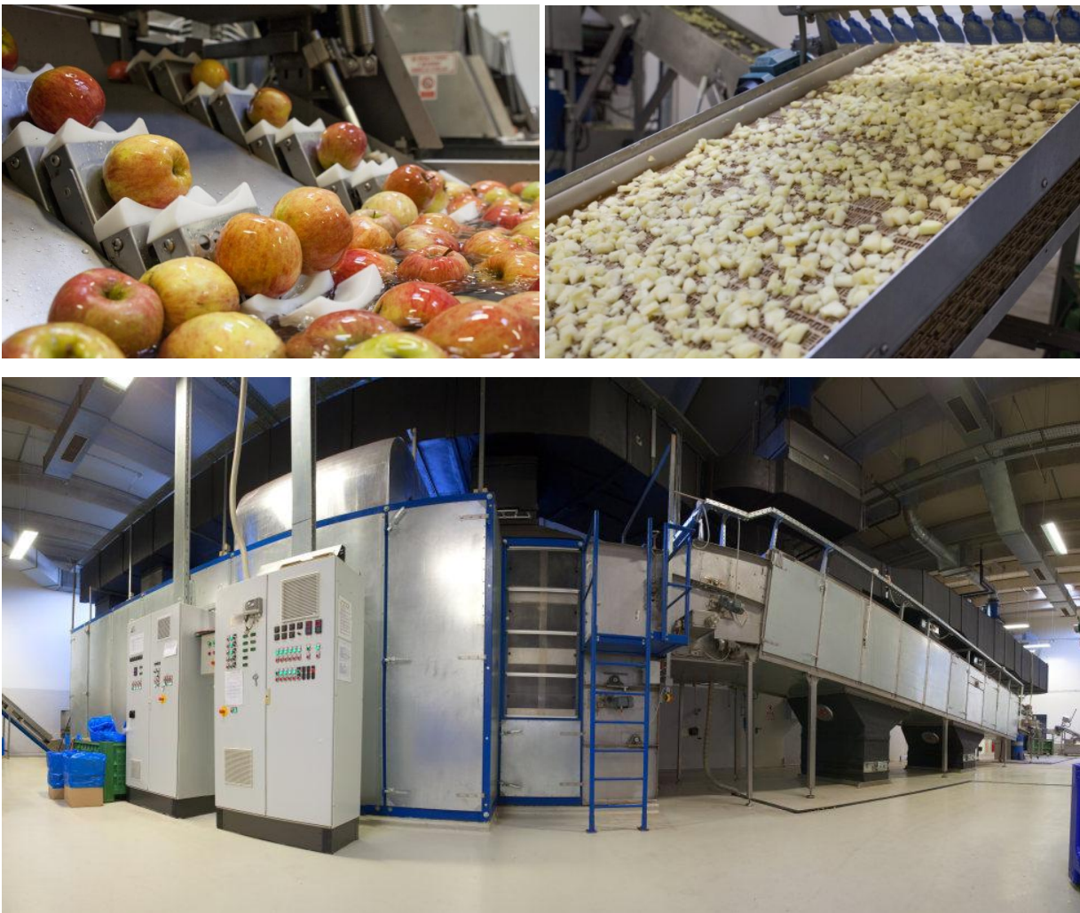
Figure 21: Production of dried apple products: top left – washing, peeling and cutting the apples; top right – apples prepared for drying; bottom – continuous drying chamber.
