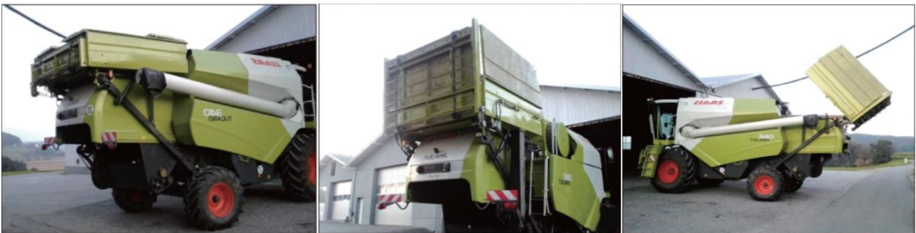
Figure 26. Maize cobs harvester with additional hopper built of divisible side walls in closed (left), opened (middle), and emptying positions (right). (Source: Dolšak B, Breznik A, Kaučič K, Imenšek N, Marčec M, Gselman P, et al. Design and initial testing of a maize cob collection system. Int J Agric & Biol Eng , 2024; 17(3): 108–114. DOI: 10.25165/j.ijabe.20241703.8218).
