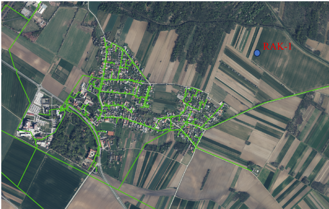
Figure 5: 20V power grid lines (green lines) and well Rak-1 (blue dot).
