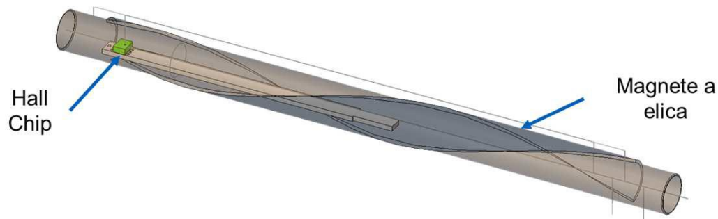
Figure 6 Detail of Hall Chip inside the transducer
