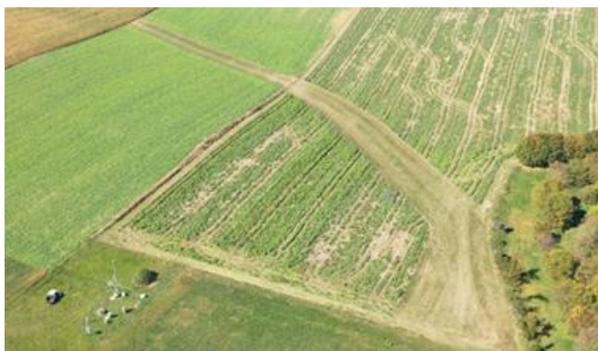
Figure 64: Grassed waterway implemented at known erosion hotspot, ©BAW-IKT
