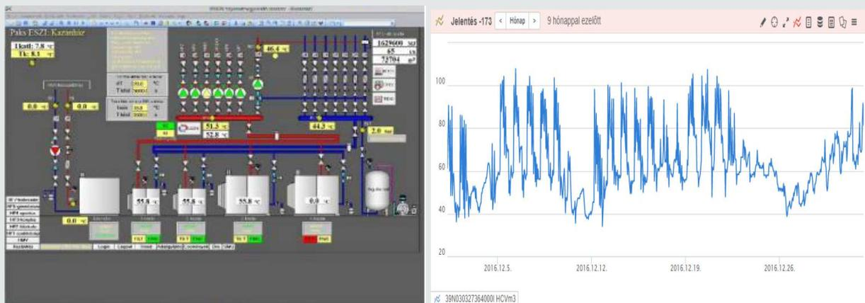
Dashboards are located in each measured buildings, usually at the entrance in order to reach the maximum possible number of persons in the building. The dashboards show the current consumption measured by the meters of the buildings (It differs from building to building: electricity is measured in all buildings, but at some buildings gas or heat consumption is also measured.). Curves of different time periods can be also visualized. The dashboards are not interactive.
