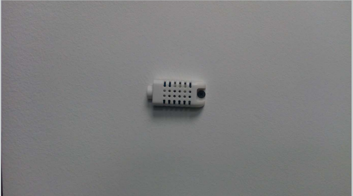
Temperature and humidity sensor
