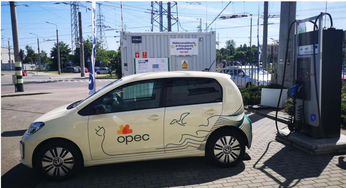
The City of Gdynia and the [trolleybus operator PKT](#) have completed two EU projects by implementing and testing an innovative solution, a mobile charging station for electric cars, powered by the trolleybus network. Within the Interreg EfficienCE project an energy storage inverter has been designed and constructed by PKT, which is a device for processing excess braking energy and traction power.
