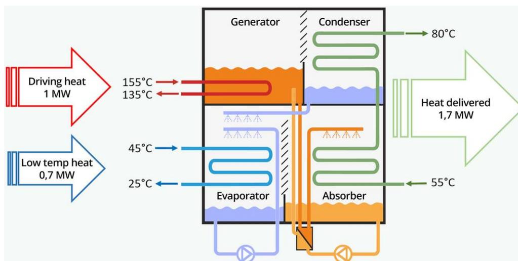
**Figure 3: Basic scheme of an absorption heat pump**
