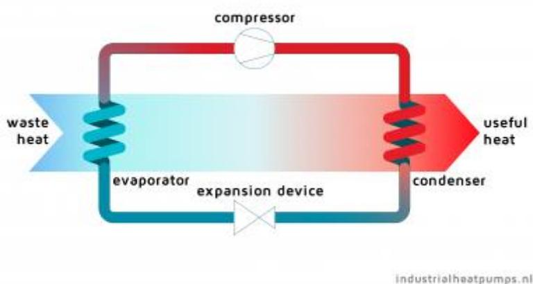
**Figure 1: Functional scheme of a compression heat pump for waste heat utilisation (source: industrialheatpumps.nl)**
