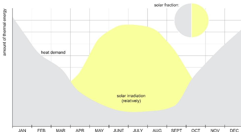
**Figure 1: Example of the radiation pattern and the heat demand of a typical DH network over one year (source: Solites)**
