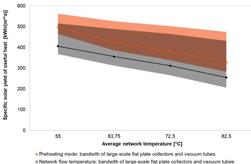
**Figure 6: Specific solar yield of useful heat from different collector types depending on the average heating network temperature and the hydraulic control integration [Quelle: Solites]**
