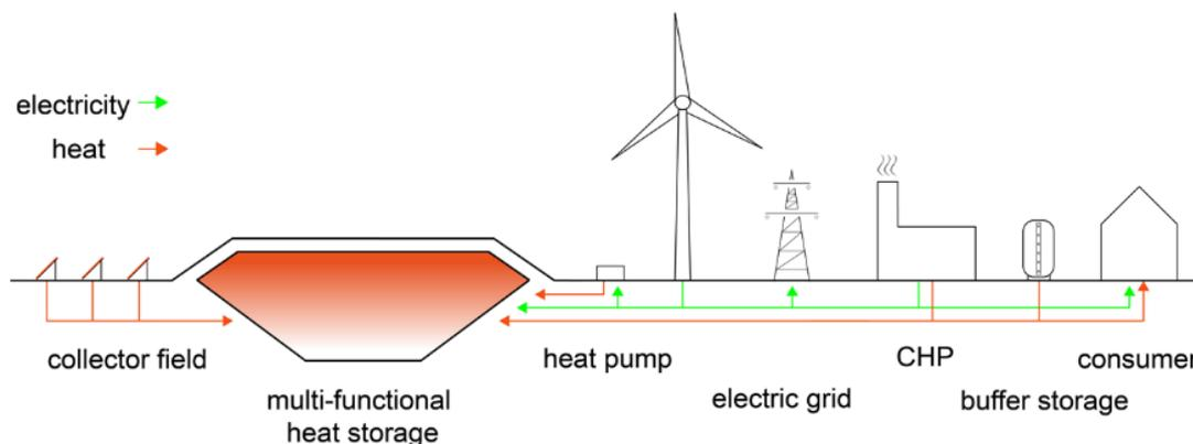
**Figure 5: Solar thermal systems are well suited for combination with other heat generation systems**
