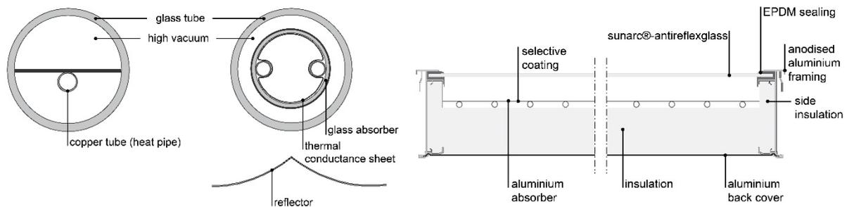
**Figure 1: Design structure of the two typical solar thermal collectors: vacuum tube collector (left) and high-temperature flat plate collector (right) [source: Solites; Wagner Solar]**
