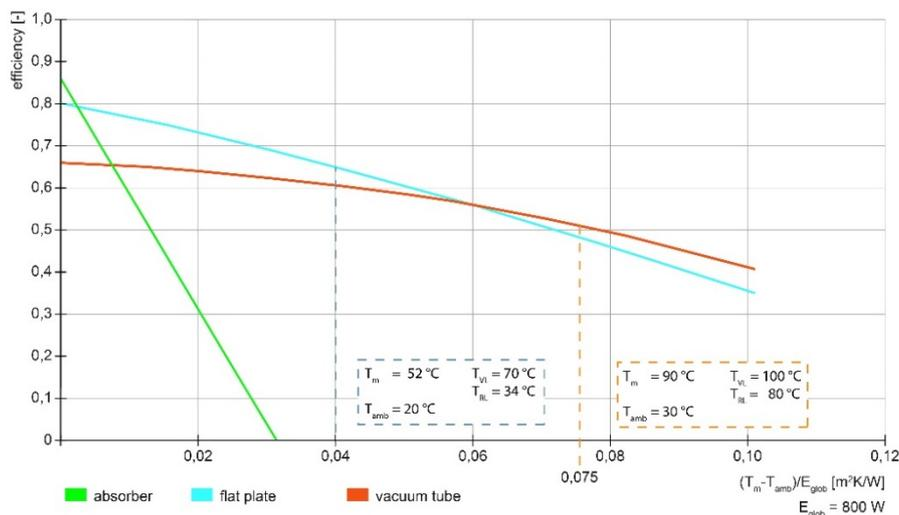
**Figure 2: Typical efficiency curves of the collector types depending on the mean heating network temperature and the outside air temperature [source: Solites]**
