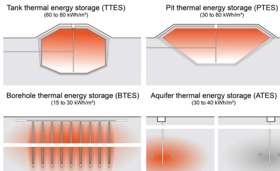
**Figure 4: Schematic representation of different storage types for long-term heat storage**
