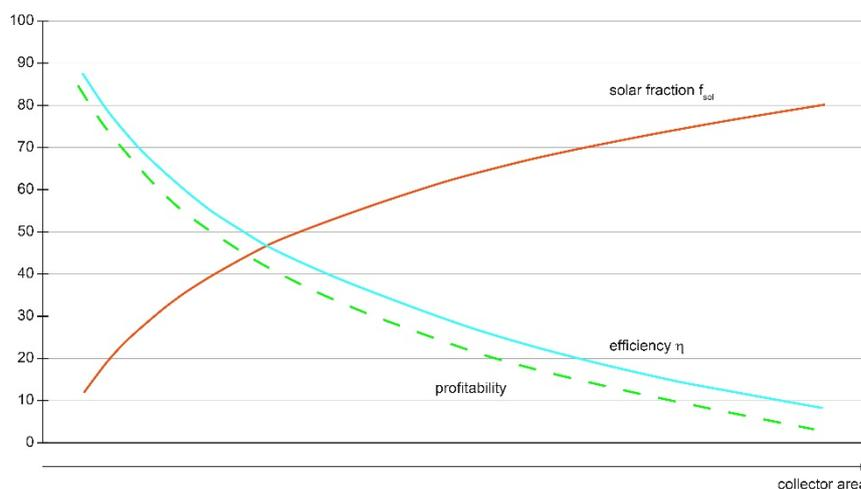
**Figure 7: Exemplary representation of the dependence of solar fraction, utilization rate and economic efficiency on the collector area [source: Solites]**
