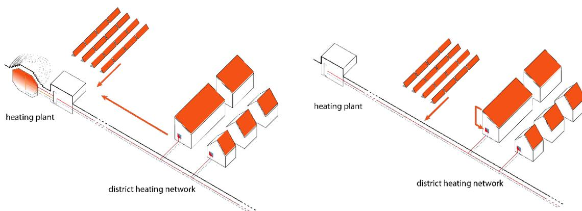
**Figure 3: Schematic representation of the centralized (left) and decentralized (right) integration of a solar thermal system in a heating network**
