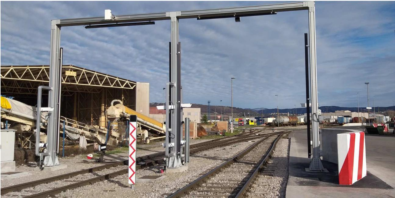
Figure 4: installed OCR system in the port of Koper (Source: Luka Koper's archive)
