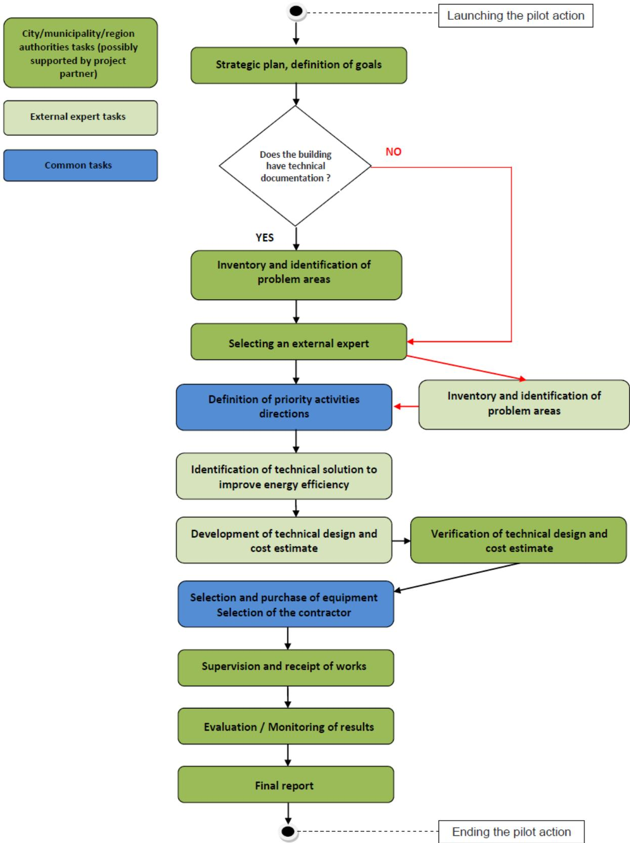
Figure 5: Traditional PA implementation procedure diagram.
