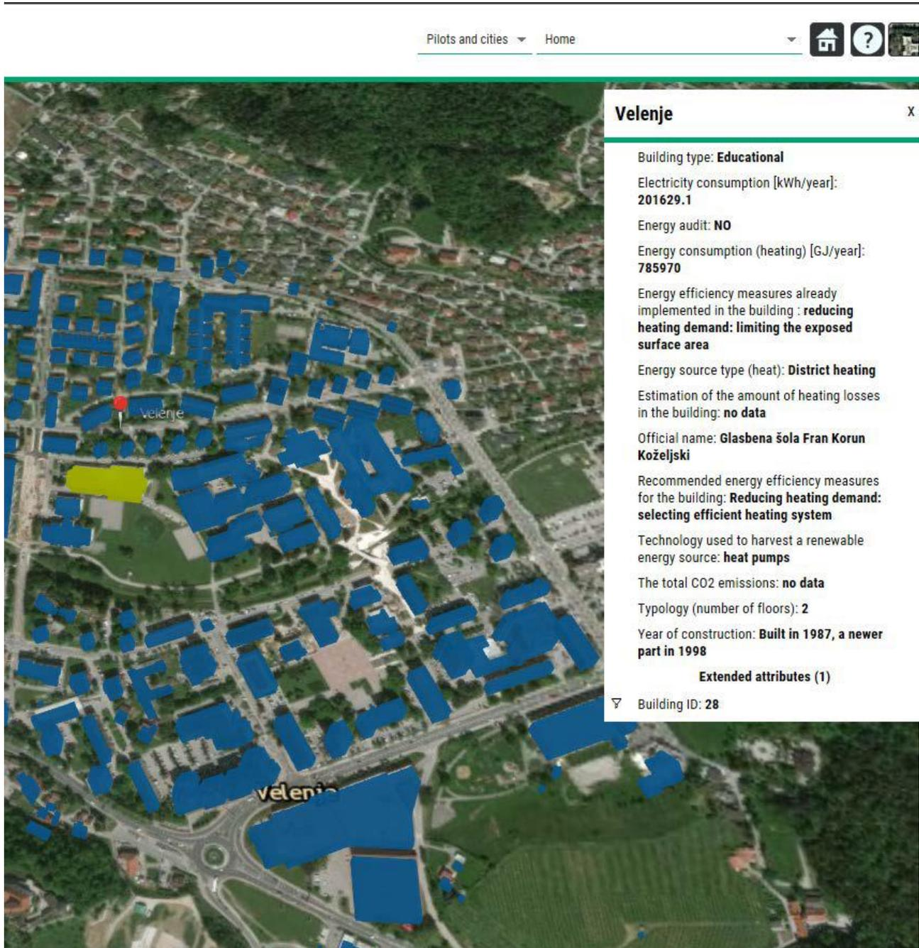
Figure 5: Pilot building in Velenje in the 3D EMS module on the OnePlace platform. Source: OnePlace platform
